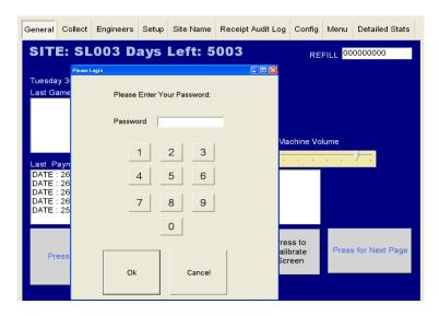
On the keyboard on the screen insert the following password to gain access to the full Engineers Menu. **000071 then Ok**
