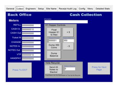
The Collect screen enables you to see the Short Term Cash In / Out meters so you can calculate how the machine is performing and this screen assists the collector to set the hopper level and also dump the hopper content.
