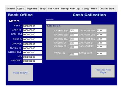
The Collect screen enables you to see the Short Term Cash In / Out meters so you can calculate how the machine is performing.
