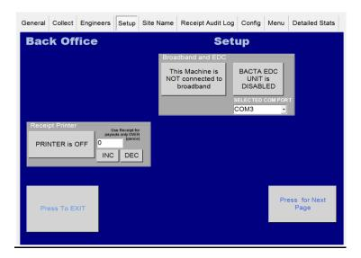
**Printer** – If a printer is fitted this allows you to turn the printer off/ on, also by pressing the **INC & DEC Icons** this allows you to choose the printer payout level the customer requires.
