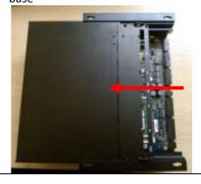
5. Disconnect the two HDD cables
